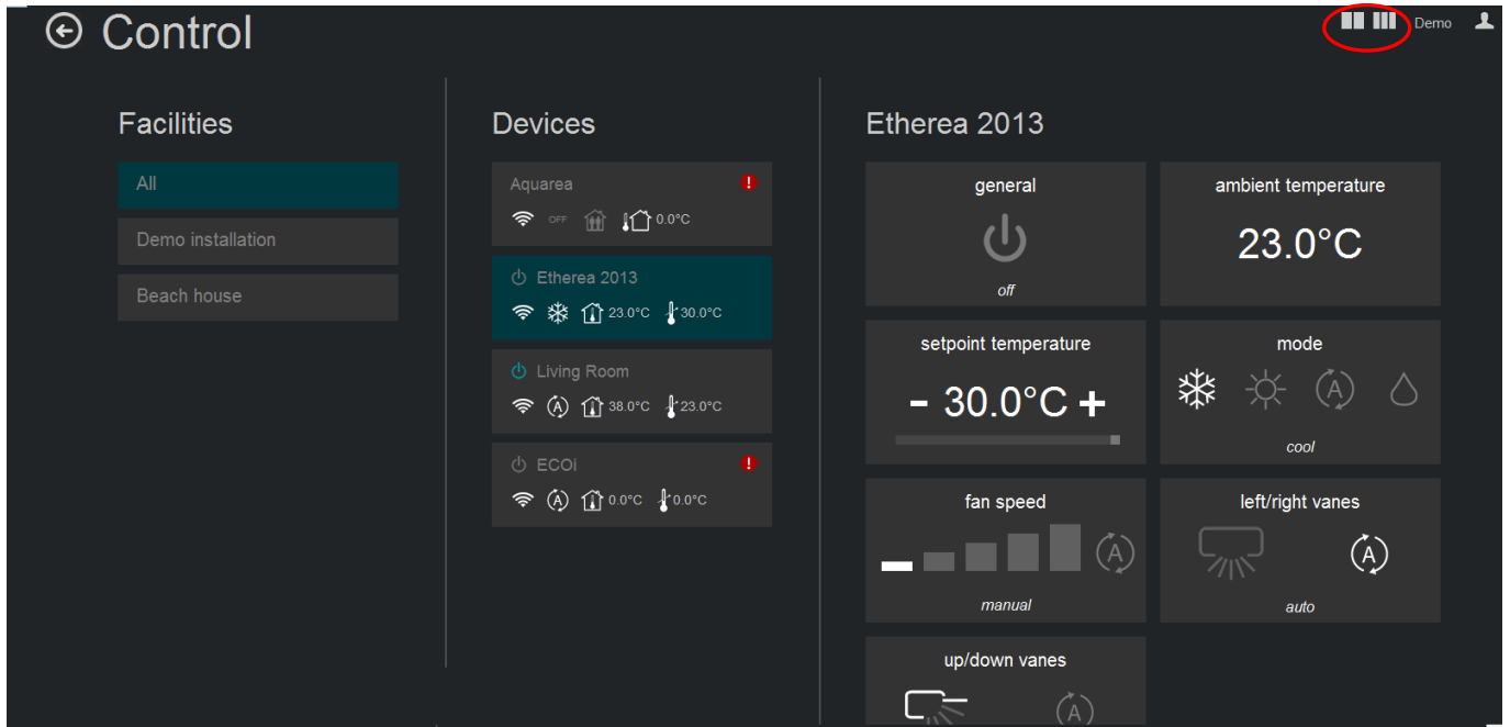
Figure 8-3 IntesisHome control interface (expanded)
